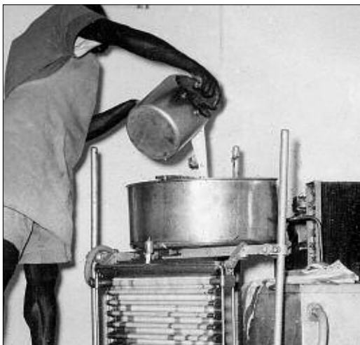
Hot milk being poured into the chiller. The milk, passing over those coils, is cooled very rapidly.
