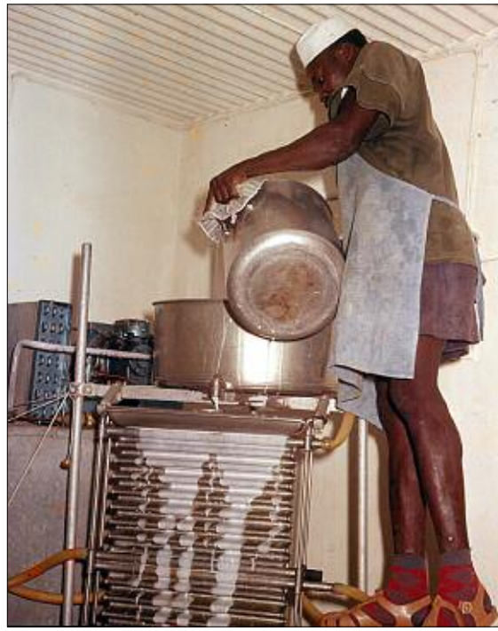
After the milk is boiled, it is chilled by means of a cooling device.
